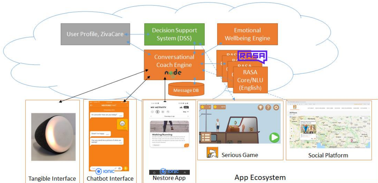
Figure 1. Architecture of WP5 interfaces with particular focus on the conversational agent and emotion engine.
