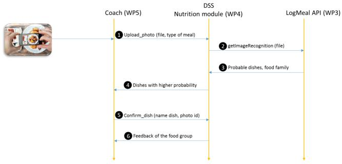
Figure 6 Communication sequence when a photo of a dish is uploaded.
