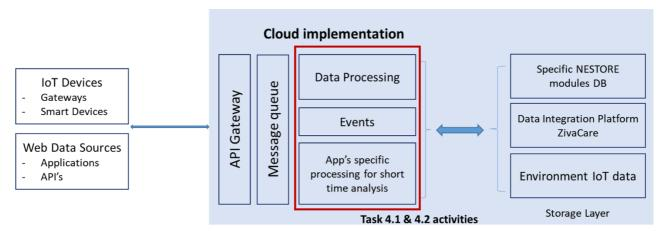
Figure 2 The data processing framework running on the NESTORE cloud infrastructure
